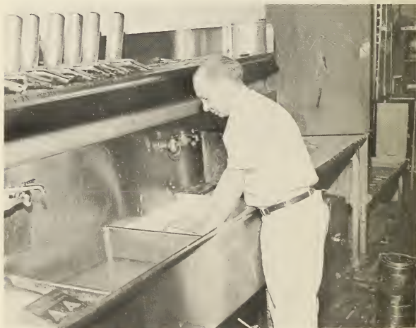
Washing and bactericidal treatment in a 3-compartment sink.
